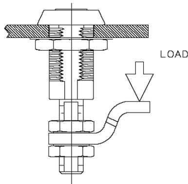
COMPRESSIVE STRENGTH - Maximum WORKING LOAD ①: 670 N / 150 LBS
